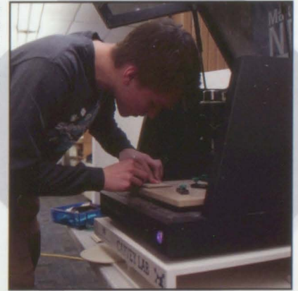
Senior Konner Kudron lines up the piece of wood with the guiders. This machine would engrave a design onto a slice of wood.
